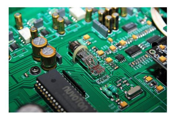
The EvolutionEVO 100 delivers an output voltage of 2V nominal and the output impedance is 2800 Ohm, which is high for loads that can drop below 10 kOhm. The output signal then decreases proportionally, the distortion does not increase at all according to PrimaLuna. This is because the 'last' tube (ECC82/12AU7) is set very far in class A bias, with the two tube halves parallel, to makes the linear area twice as large.
